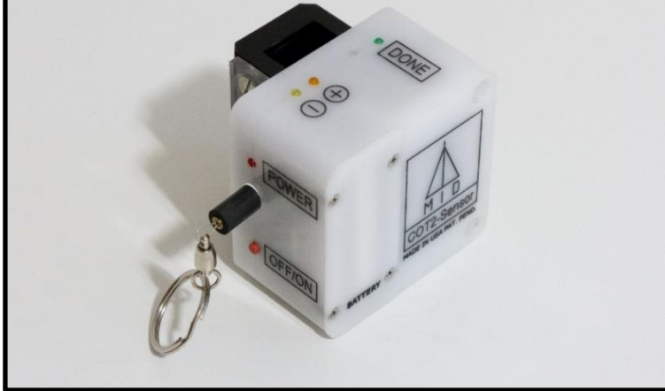
COT-Sensor (placed at each installed bracket)
