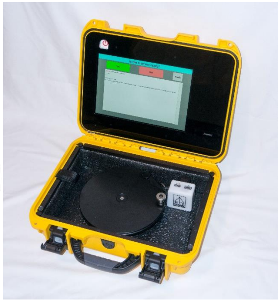
COT4- Controller (wireless, battery operated)
